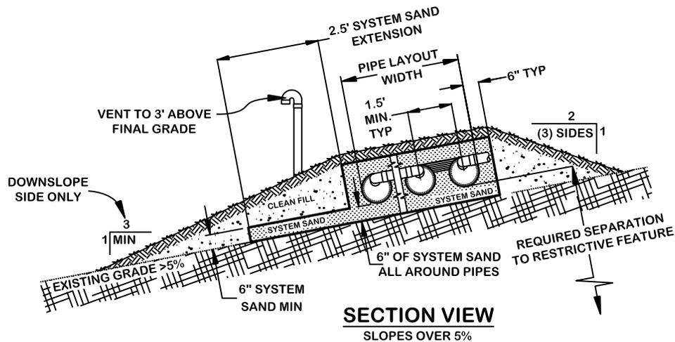
Figure 3-20. Advanced Enviro Septic® System Treatment Components.
