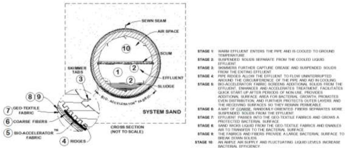
Figure 3-21. Advanced Enviro-Septic Pipe Design: 10 Steps of Treatment.
